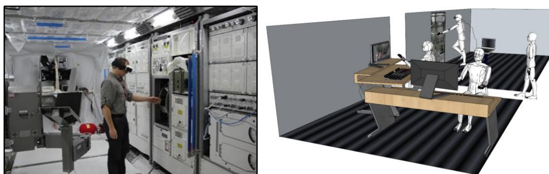
Fig. 3: Trainee wearing a HMD inside ISS/Columbus mock-up (left) and interaction relationships between the actors of the training/simulation process (right).
